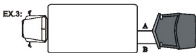
EX.3: Distance A will be detected first, and then distance B be detected when the car reverse close.
