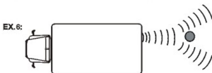
EX.6: The system may not detect a small and smooth round pole.
