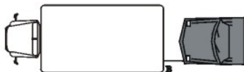
However, as the car reverse closer, A may fall into the sensor's blind zone. In such cases, the system will misjudge B as the closest distance.
