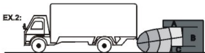
EX.2: Complex environment: B and C will be detected but A cannot be detected.
