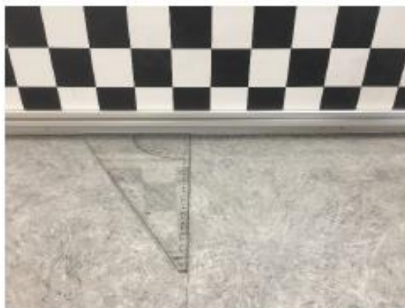
Finding a line perpendicular to the wall
