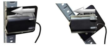
Example of horizontal antenna mounting (arrow pointing in the direction of travel> front of the car):
